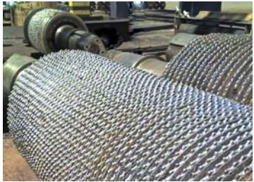
Hardfacing can be used on cane rolls to create a hook profile to increase productivity as well as increasing service life up to 300% or more.
