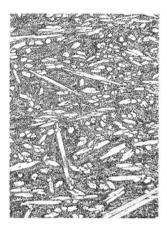
Hardfacing alloys consist of several materials. This micrograph shows a chromium carbide high-alloy type magnified more than 50 times.
